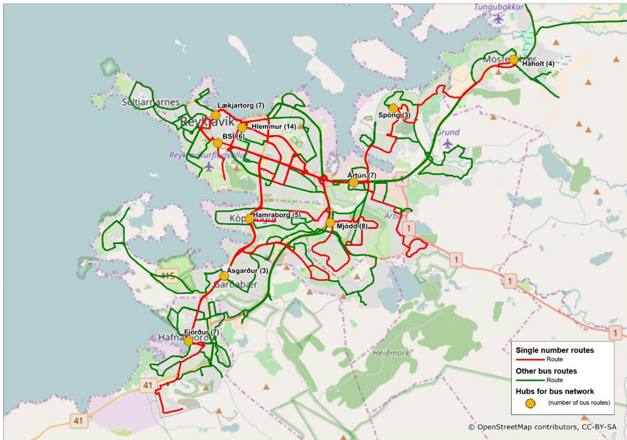
Figure 13 Existing bus network – shown as "single number" bus routes and other bus routes. Furthermore, hubs are shown with number of bus routes serving the hub.
